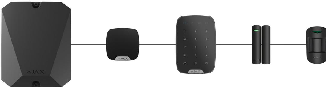
When using the **Beam (Radial) topology**, be sure to install a 120 Ohm terminating resistor at the end of the line (included in the hub complete set). The terminating resistor is connected to the signal terminals of the last detector on the line.
