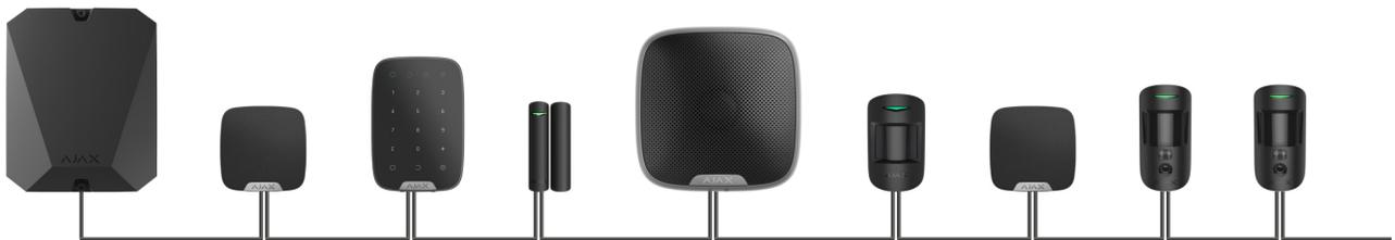
**Ring connection** takes two bus outputs of the hub. If the ring breaks in one place, no device will be disabled. The ring reconfigures into two lines, which continue to operate normally. Users and security company will receive notification about the break.
